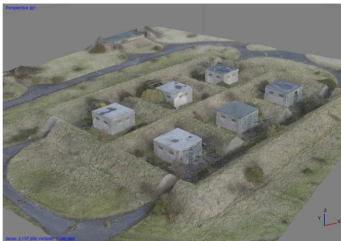
Example of a shaded DSMs created using AGISOFT Photoscan
